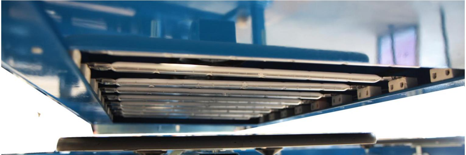
The COSMOTEX flash combines the action of the halogen quartz lamps with emission of short wave infrareds and the air, increasing their effectiveness.
