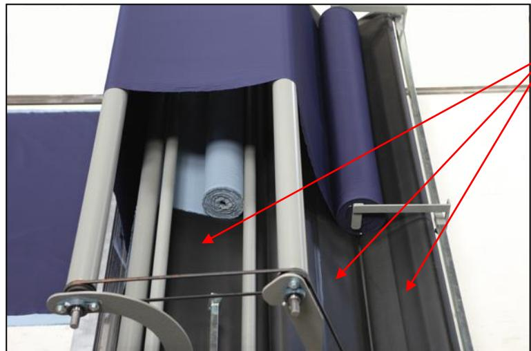
**NEW SYSTEM FABRIC UNWINDS FOR HEAVY ROLLS:** Apolo Smart has an innovative system of REINFORCED cradle with three belts where speeds can be adjusted independently by inverters. Synchronization between a double band cradle and the single delivery belt allows a perfect fabric unwinding.
